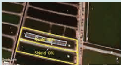
Fig. 1. The comparison of milkfish culture ponds with simulated floating solar photovoltaic between Shield rate 40% and Shield rate 0% at 23°07'24.41"N 120°04'49.67"E. (From google maps).
