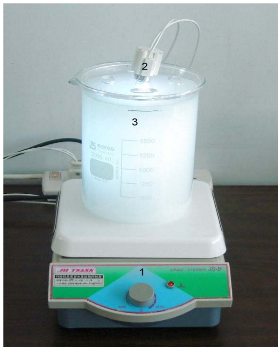
Fig. 1 Experimental setup. 1. magnetic stirrer; 2. UV-A lamp; 3. beaker.
